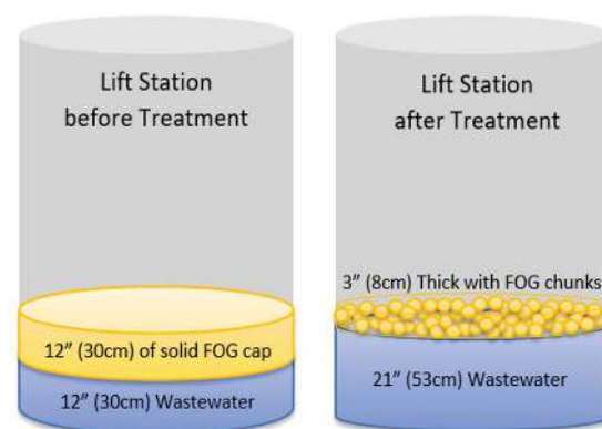
Figure 1: Solid FOG cap prior to treatment (left), digested & liquefied FOG cap after two months of treatment (right)
